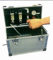
④ Open valve. When reading is stable store the measurement to memory
