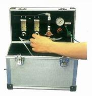
3 Adjust flow to the specified rate using flowmeters A & B
